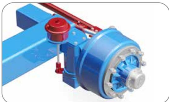
Pneumatic breaking with brake chamber
